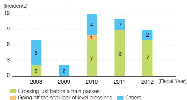
Accidents at level-crossings
